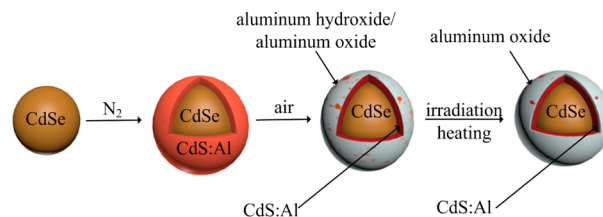
Figure 5. Schematic illustration for transformation process from aluminum hydroxide to aluminum oxide.
